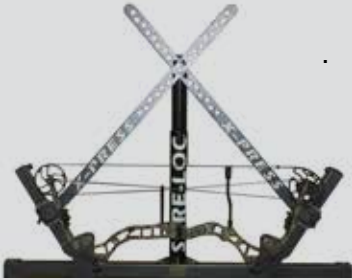
FIG. 1 PRESSES BOW IN TWO PLACES
